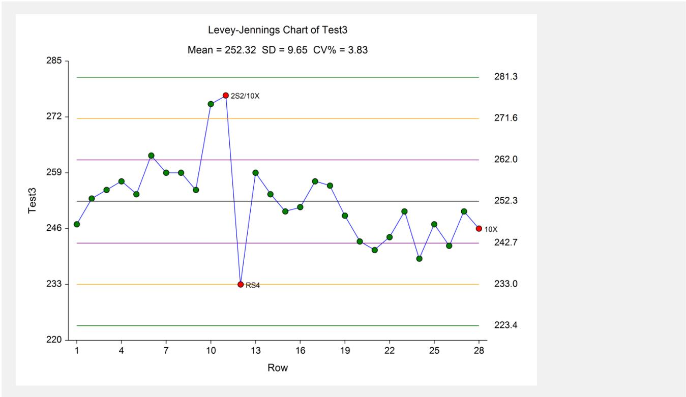
This plot displays the Levey-Jennings control chart. The overall mean (center-line) and three sets of control limits are shown. Notice that three rows are out of control. The next report gives the numerical details of the charts and lists those rows that failed at least one of the control tests.
