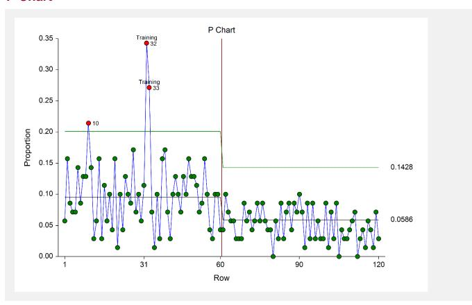
The P chart shows the substantial decrease in the proportion of leaking connections in the second stage. The center line and limits of the second stage are estimated from samples 61 to 90.
