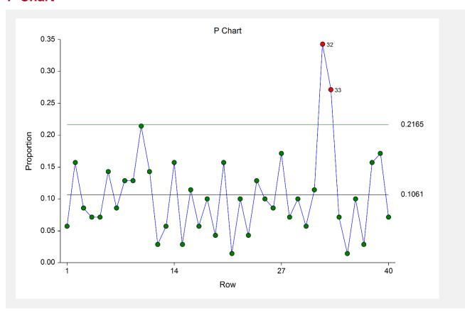
The P chart shows the sequence of proportions of leaking connections. The chart show that samples 32 and 33 merit further investigation for an assignable cause. After reviewing the records, the investigators found that the 32<sup>nd</sup> and 33<sup>rd</sup> samples came during and immediately after the training of a new connection installer.
